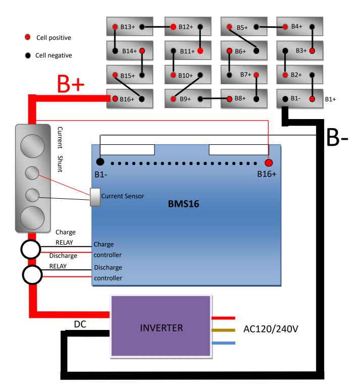
Heavy RED wires are positive of battery pack (B+/B16+), charger and load such as motor, and heavy black wire is negative of battery pack(B-/B1-), charger and load.
